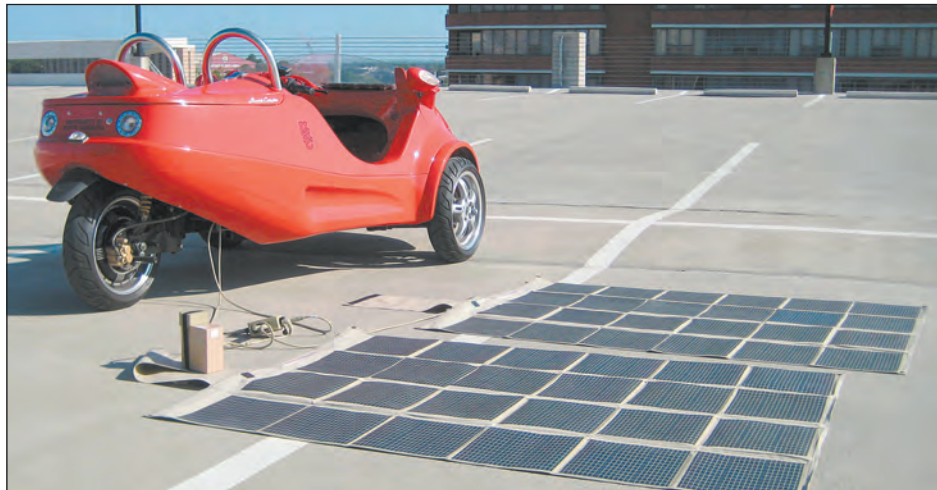
To assist with charging the main batteries, a 120W flexible foldable solar panel can be deployed on sunny days to acquire a 10-15% charge on the 48V 36Ah main battery system
