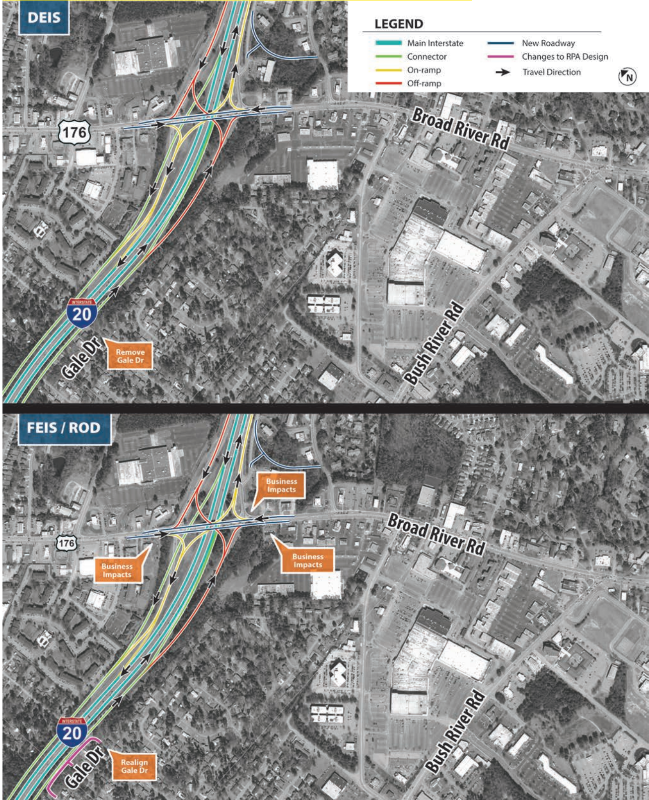
Figure 7D Design changes to RA1 – I-20/Broad River Road and Gale Drive Alignment
