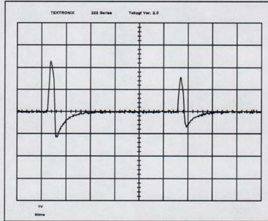
Roadtrax BL Sensor taped to the road. 12' long with 100' passive cable. Chevy Caprice = 25 mph. 4/25/96. 1V/div vertical scale; 50 msec/div horizontal.
