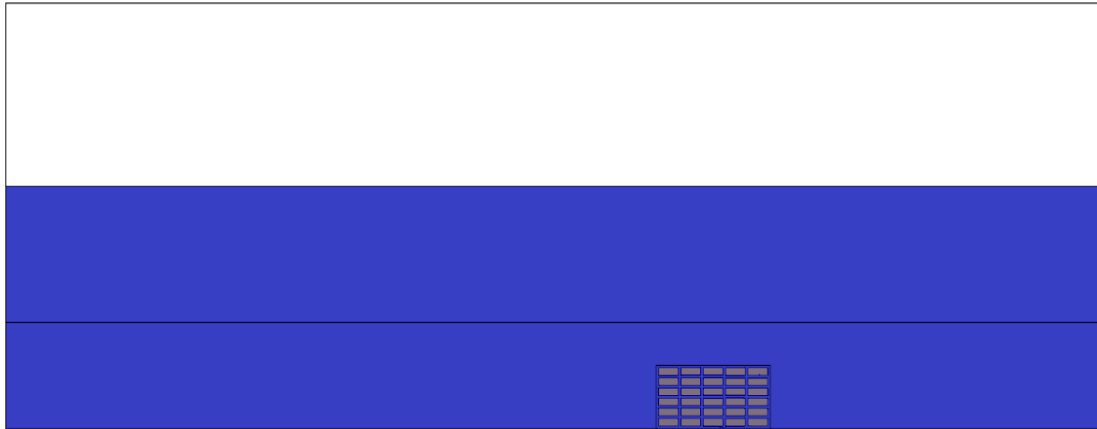
Figure 3-2: The full width of the shoulder and the 12 ft roadway lane (black edges), and the part chosen as the computational domain (dark blue)
