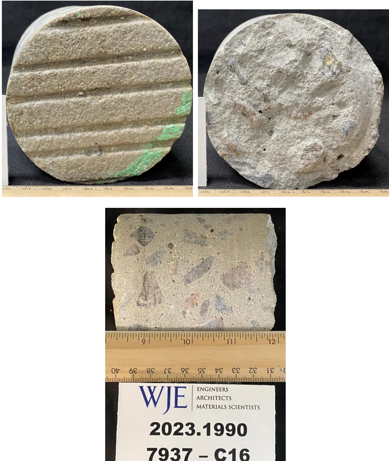
Figure 10. 7937-C16. As-received, with the top surface in the top left image, bottom surface in the top right, and a longitudinal view of the core with the top surface to the left in the bottom image. Note the very well-preserved tines and slightly glossy or shiny appearance on the top surface.
