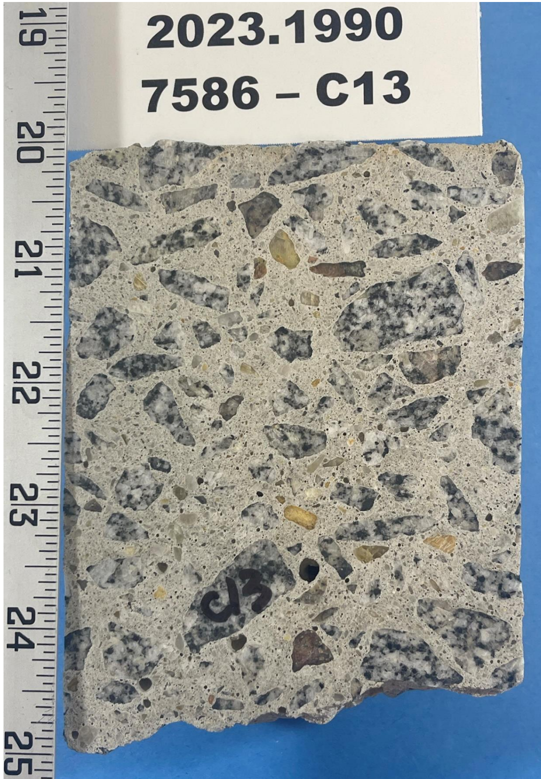
Figure 23. 7586-C13. Lapped longitudinal section, with the top surface towards the top of the image. Note the uneven top surface and loss of fines. The aggregate in cores from Asset 7586 is different than that from 7272.
