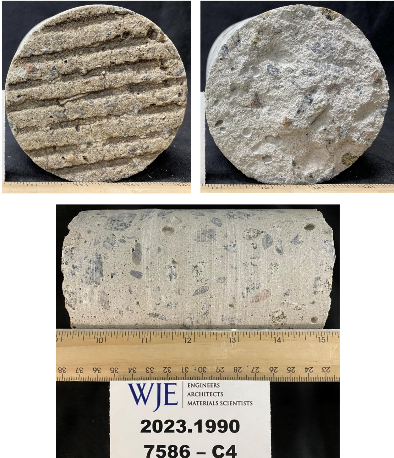
Figure 5. 7586-C4. As-received, with the top surface in the top left image, bottom surface in the top right, and a longitudinal view of the core with the top surface to the left in the bottom image. Note the well-preserved tines on the top surface.
