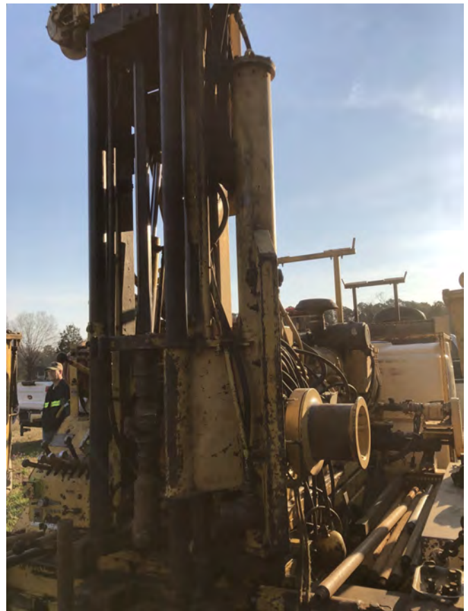
Figure No. 4: Automatic Hammer
