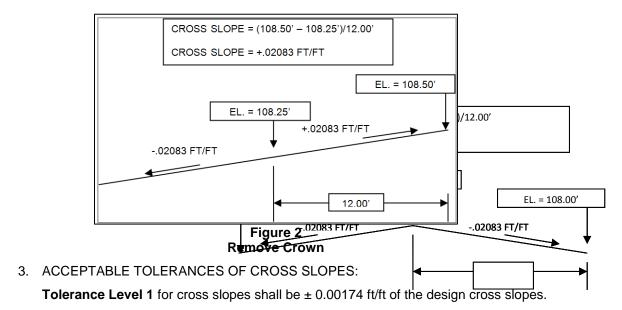
**Tolerance Level 2** for cross slopes shall be  $\pm 0.00348$  ft/ft of the design cross slopes.
