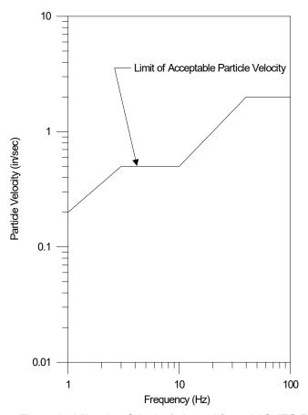
Figure 1 - Vibration Criteria (adapted from AASHTO R8-96)
