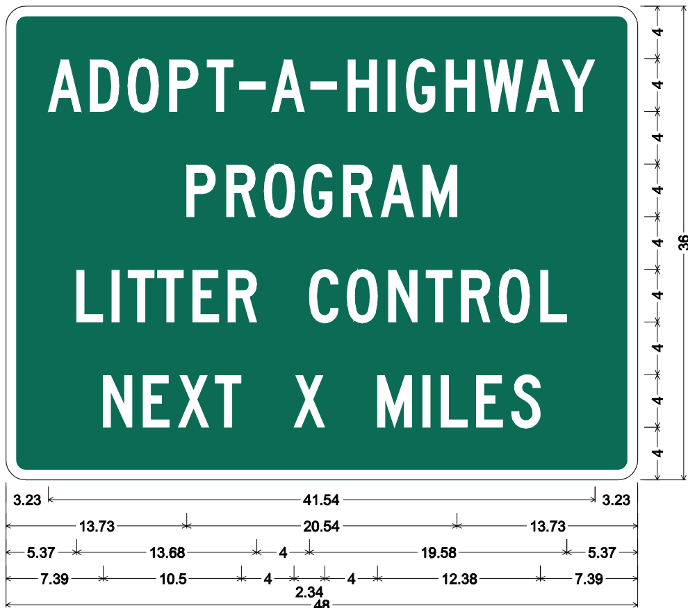
I-10-1-48; 1.50" Radius, 0.75" Border, White on Green; [ADOPT-A-HIGHWAY] C; [PROGRAM] C; [LITTER] C; [CONTROL] C; [NEXT] C; [X] C; [MILES] C;
