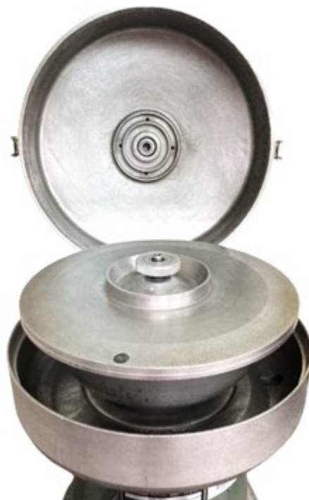
Figure 3: Inside the centrifuge extractor, depicting the bowl unit with lid and nut
