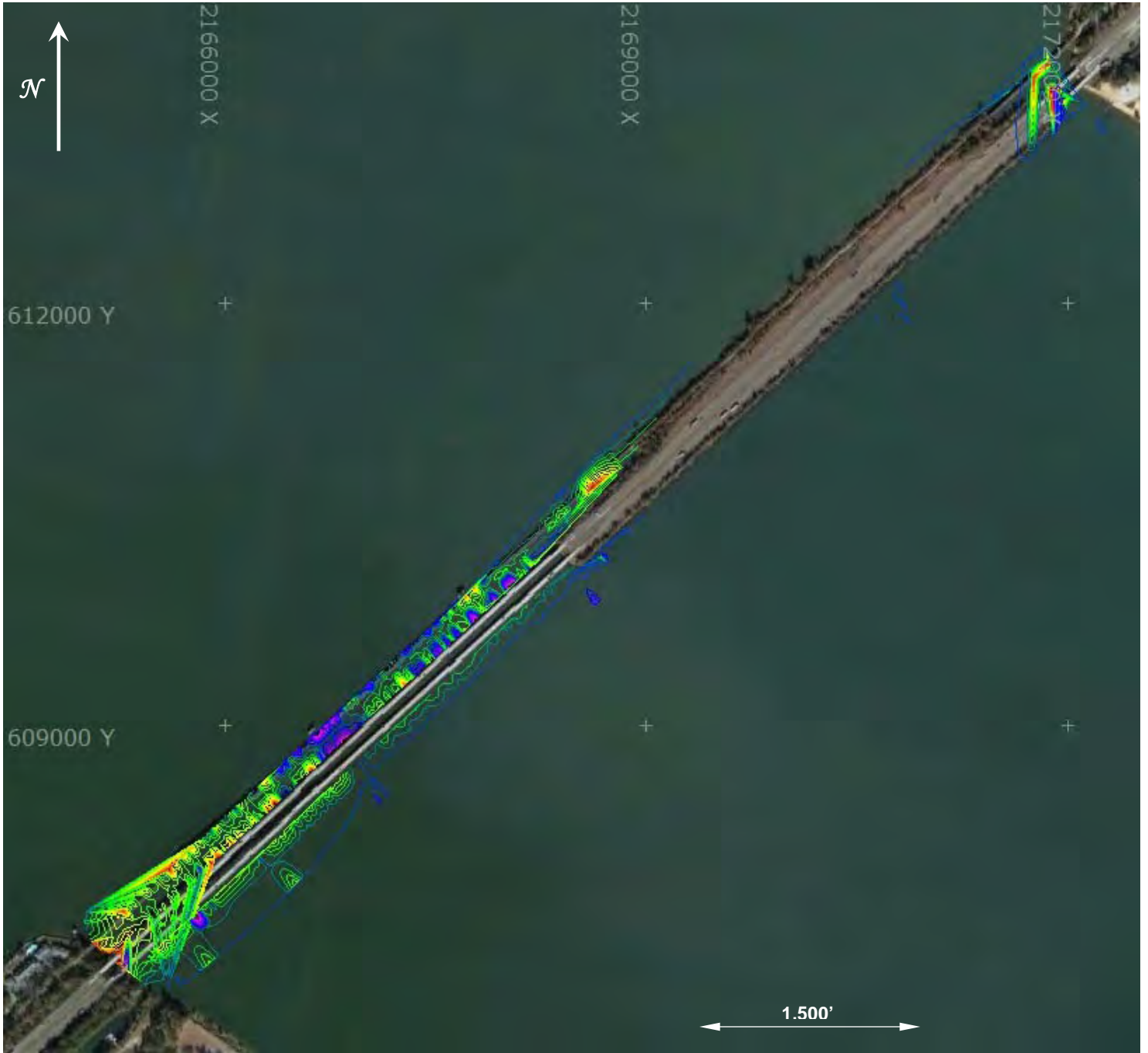
Figure 6. Magnetic Contours at 300 nT (gamma) Intervals at Lake Marion Project Area overlaid on an Aerial Photograph
