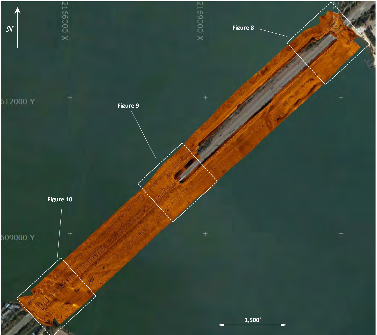
Figure 4. Sonar Mosaic of Lake Marion Project Area overlaid on an Aerial Photograph
