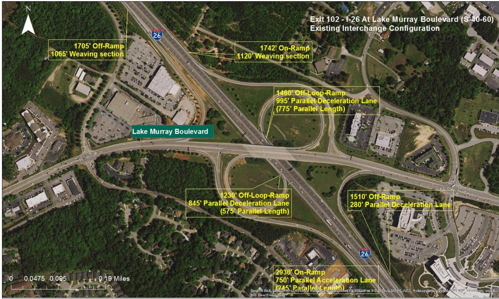
Figure 35 - Exit 102: Existing Interchange Configuration
