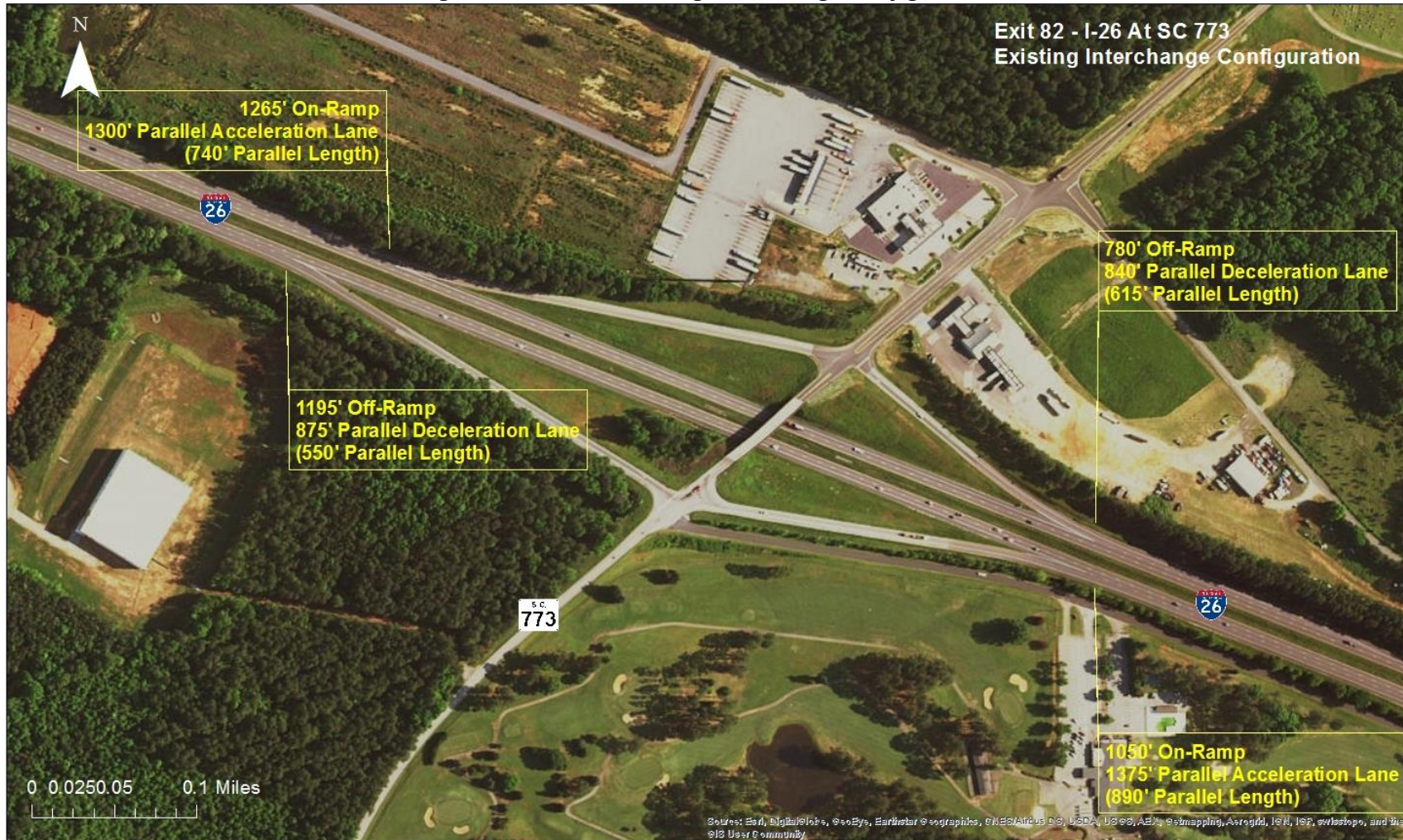
Figure 8 - Exit 82: Existing Interchange Configuration
