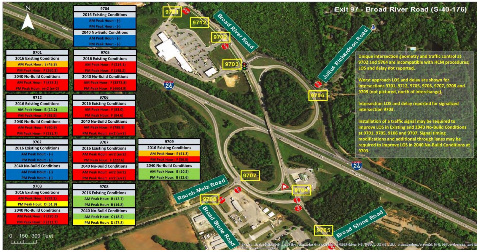
Source: Figure 76, Interstate 26 Widening Traffic Analysis Report Figure 18. Exit 97 – Broad River Road (US 176) Interchange Intersection LOS Summary
