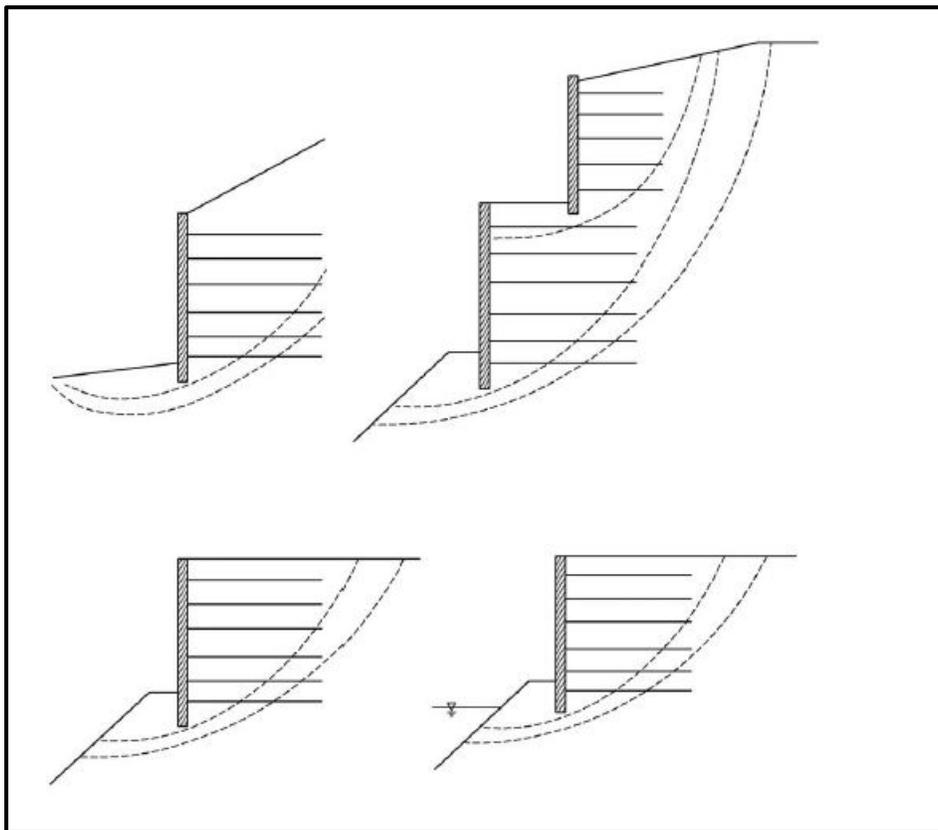
**Figure C-22, Compound Stability MSE Wall Geometries
