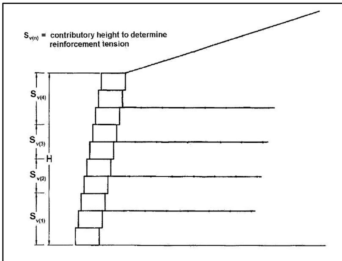
**Figure C-12, Reinforcement Load Contributory Height
