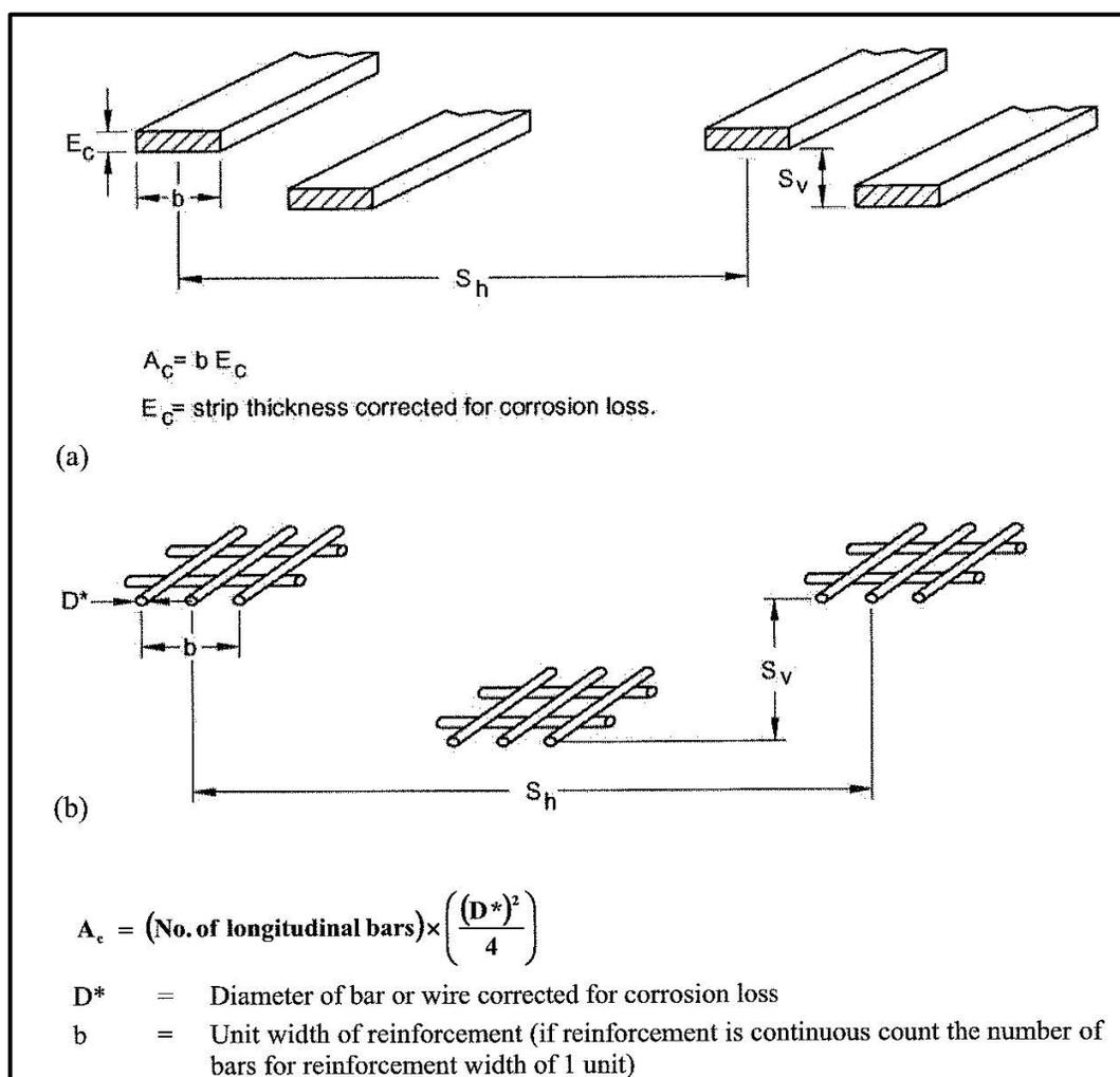
**Figure C-14, Geometric Configuration of Metallic Reinforcement
