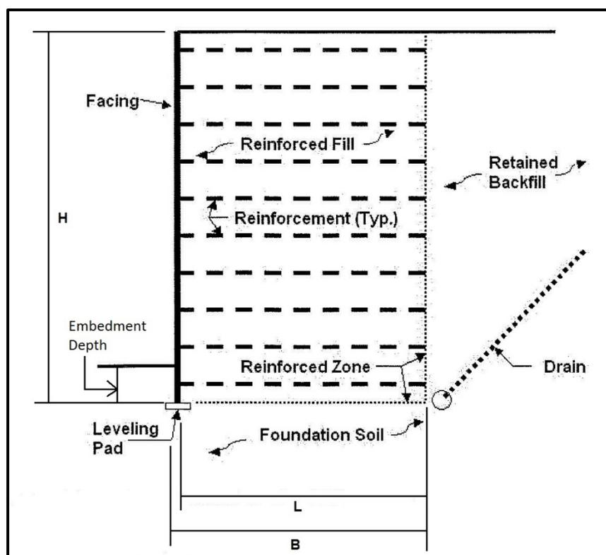
**Figure C-1, General MSE Wall Schematic
