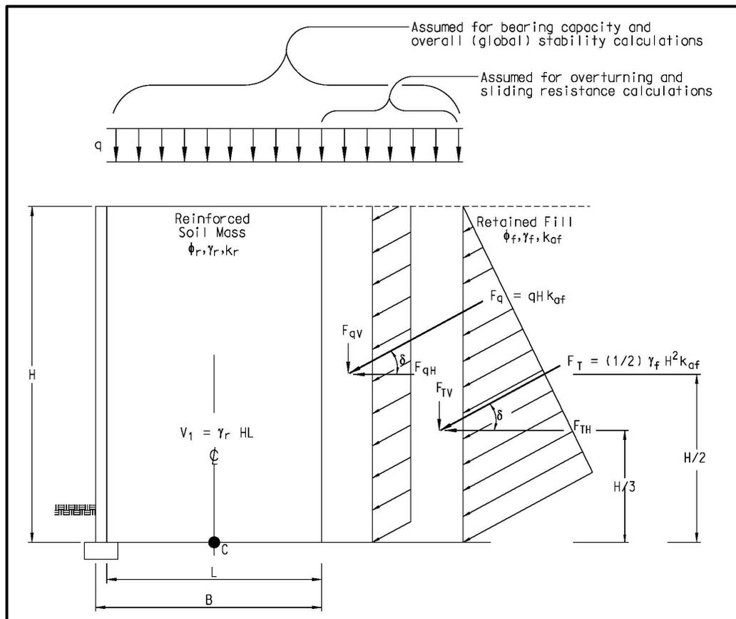
**Figure C-2, MSE Wall Earth Pressure for Horizontal Backslope
