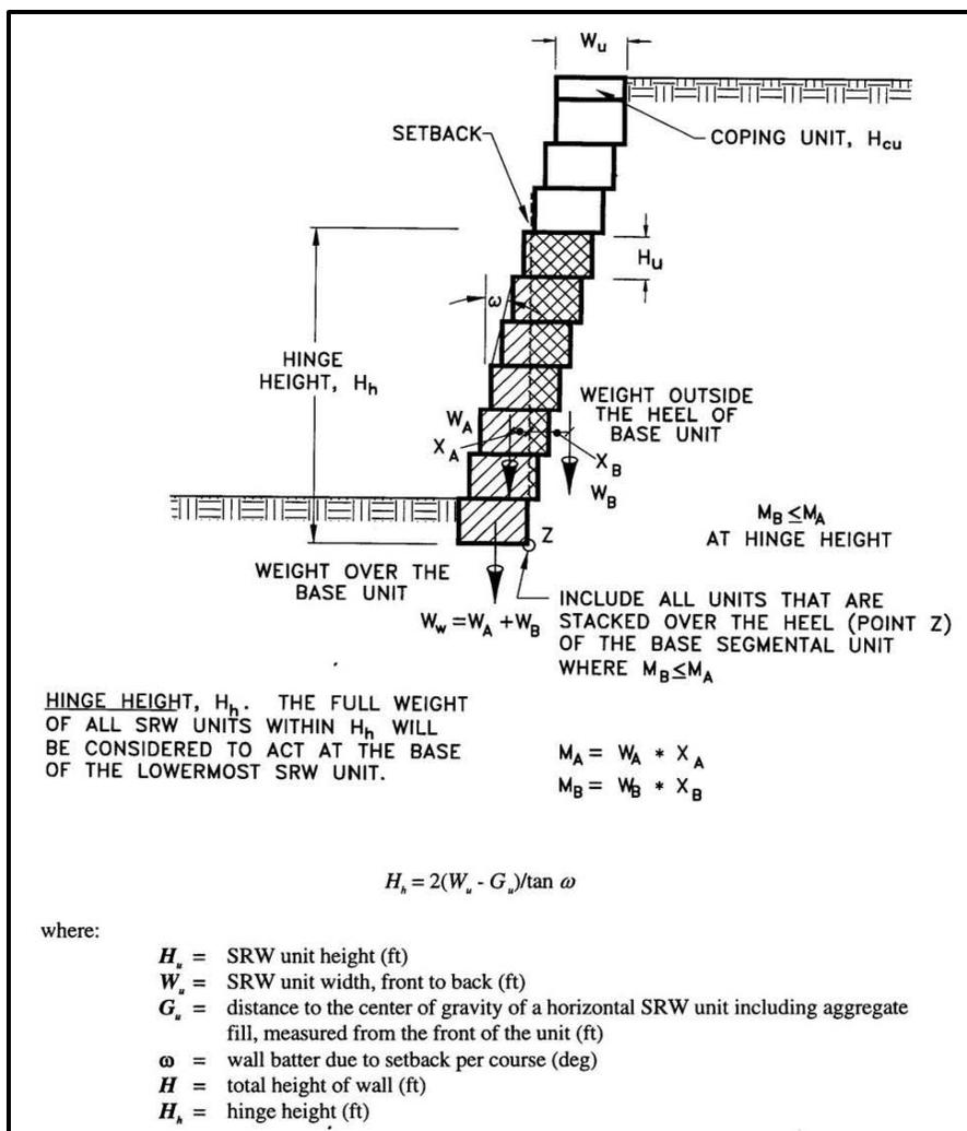
Figure C-20, Hinge Height of Modular Block MSE Walls
