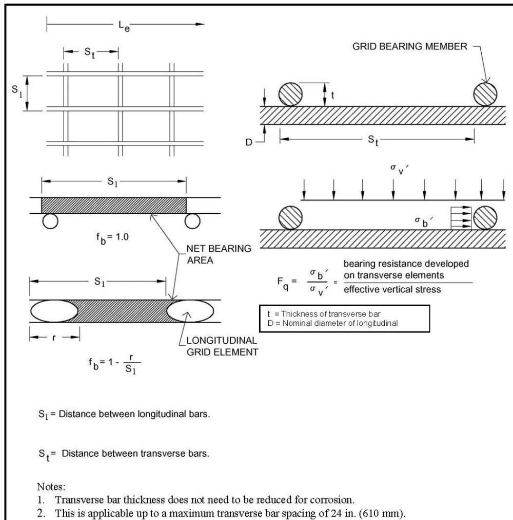
**Figure C-18, Grid Dimensions for Pullout Capacity
