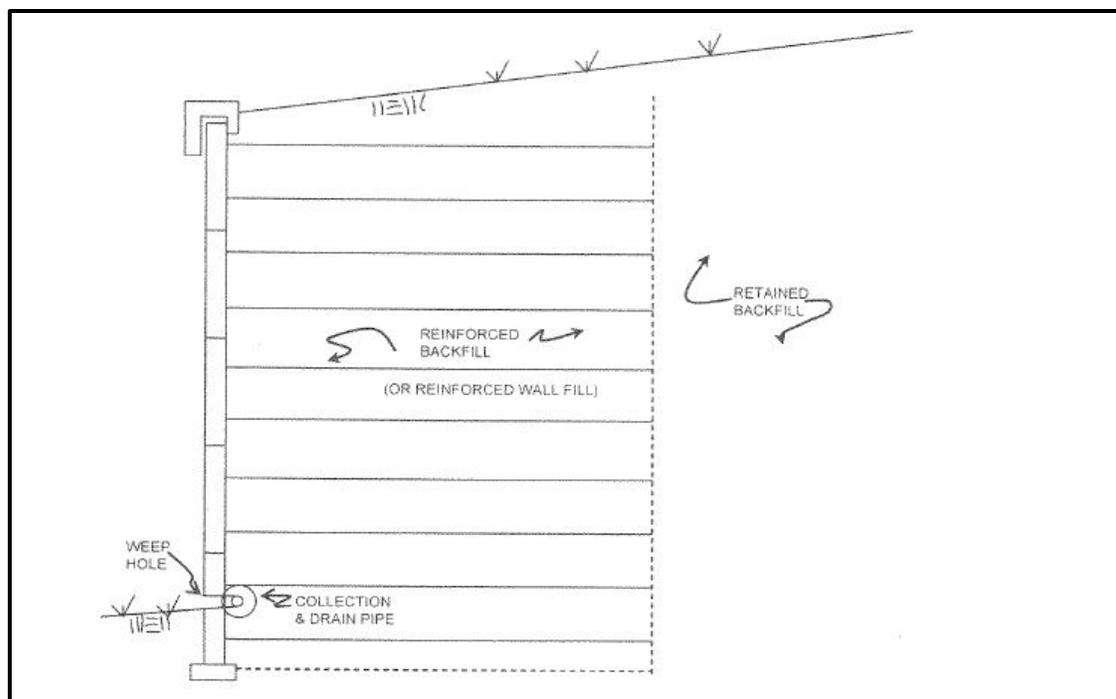
**Figure C-23, Drain Immediately Behind MSE Wall Face
