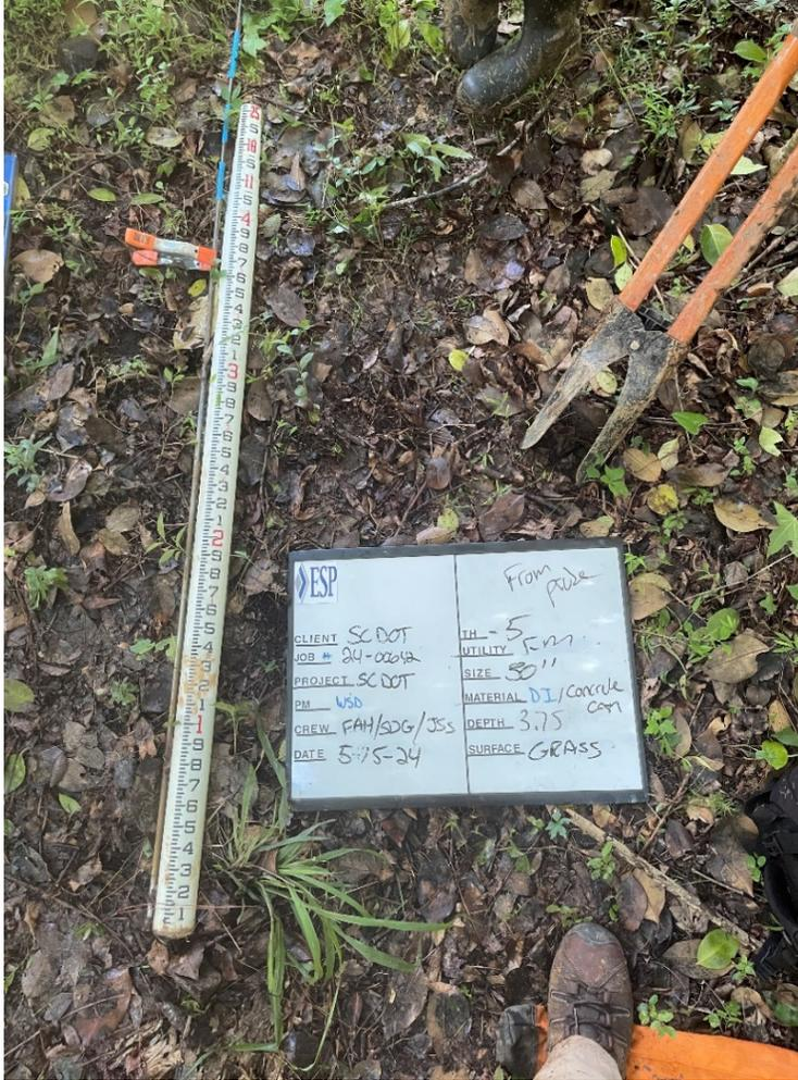
Coordinates for this survey based on SC State Plane NAD83, NAVD88 datums. Horizontal and vertical accuracies are consistent with standards set forth in the SUE standard ASCE 38-22.
