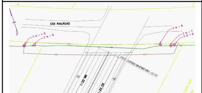
Coordinates for this survey based on SC State Plane NAD83, NAVD88 datums. Horizontal and vertical accuracies are consistent with standards set forth in the SUE standard ASCE 38-22.
