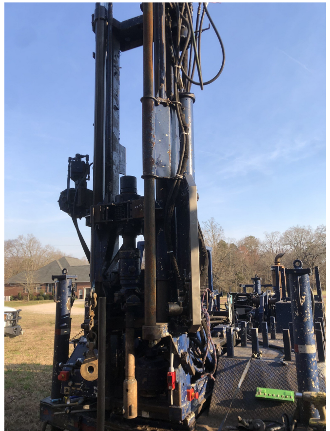
Figure No. 4: Automatic Hammer
