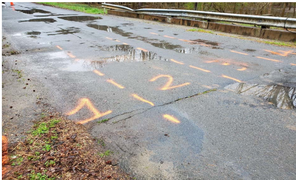
Figure 14: Temporary Marking Lines on the Bridge Deck for Proper Truck Alignment During the Load Test
