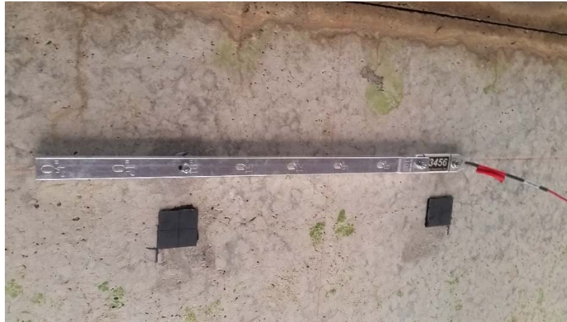
Figure 4: ST350 Strain Transducer with 24-in. extension arm.
