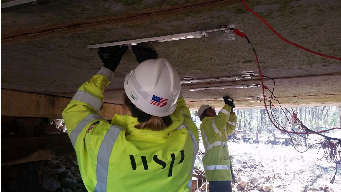
Figure 7: Strain Gauge Installation
