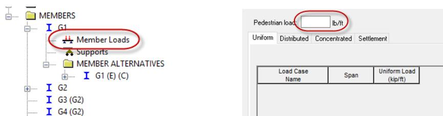
Note: pedestrian loading shall be applied similar to other superimposed composite dead loads (i.e., distributed equally to the nearest 3 girders under the sidewalk).
