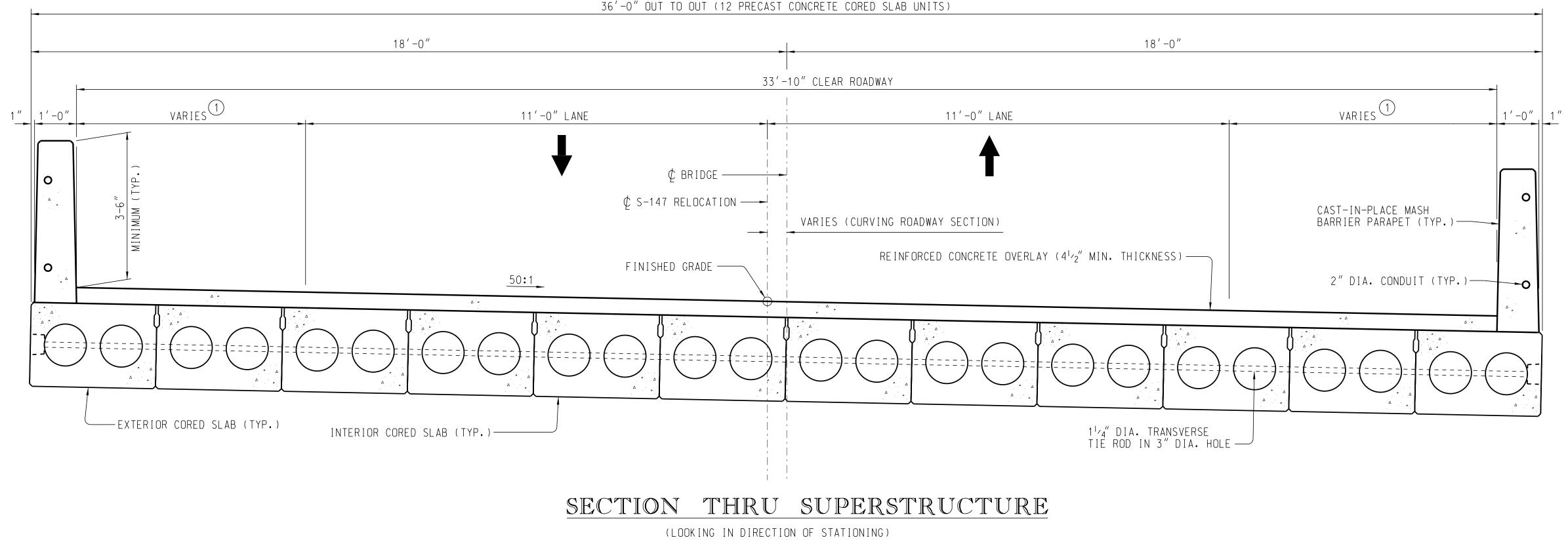
36'-0" OUT TO OUT (12 PRECAST CONCRETE CORED SLAB UNITS)
