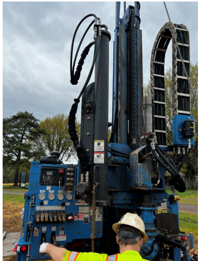
Figure No. 4: Automatic Hammer
