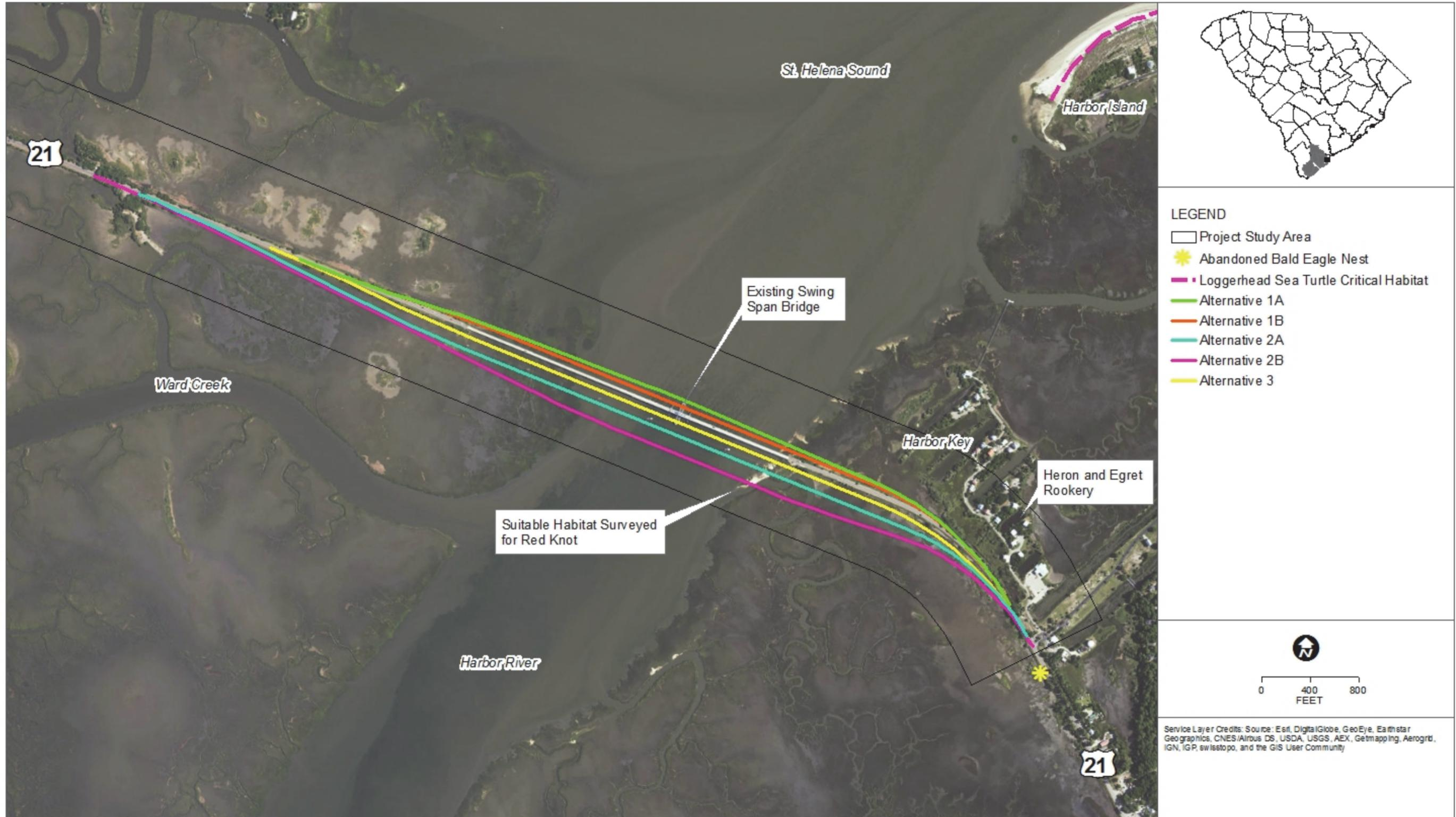
Figure 4-1. Alternative Alignments of Proposed US 21 Bridge
