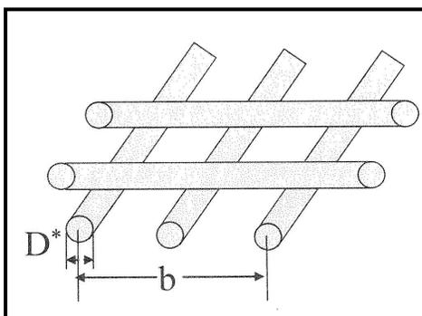
**Figure D-4, Cross Section Area for Bars
