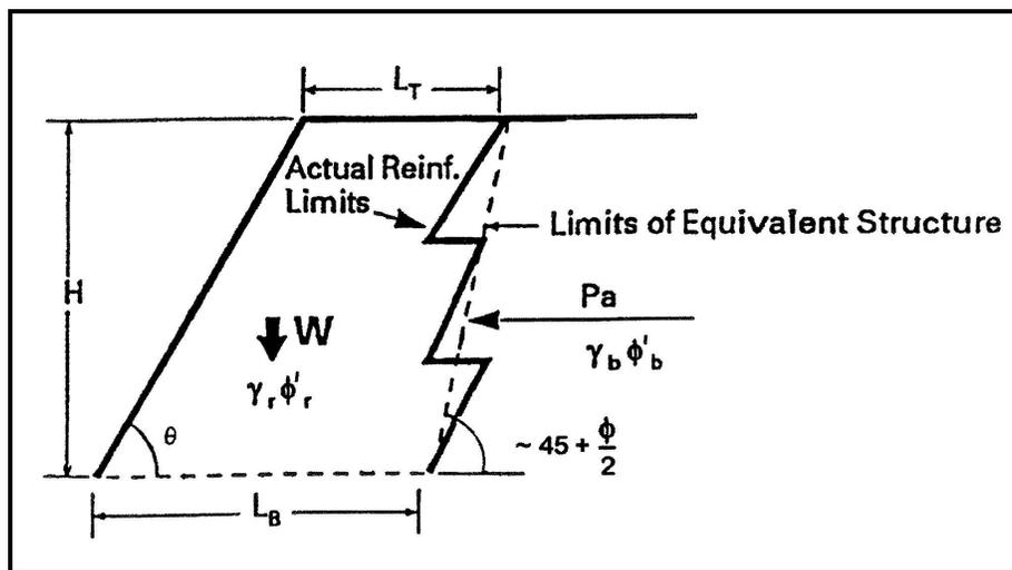
**Figure D-12, Sliding Stability Analysis
