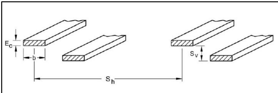
**Figure D-3, Cross Section Area for Strips**
