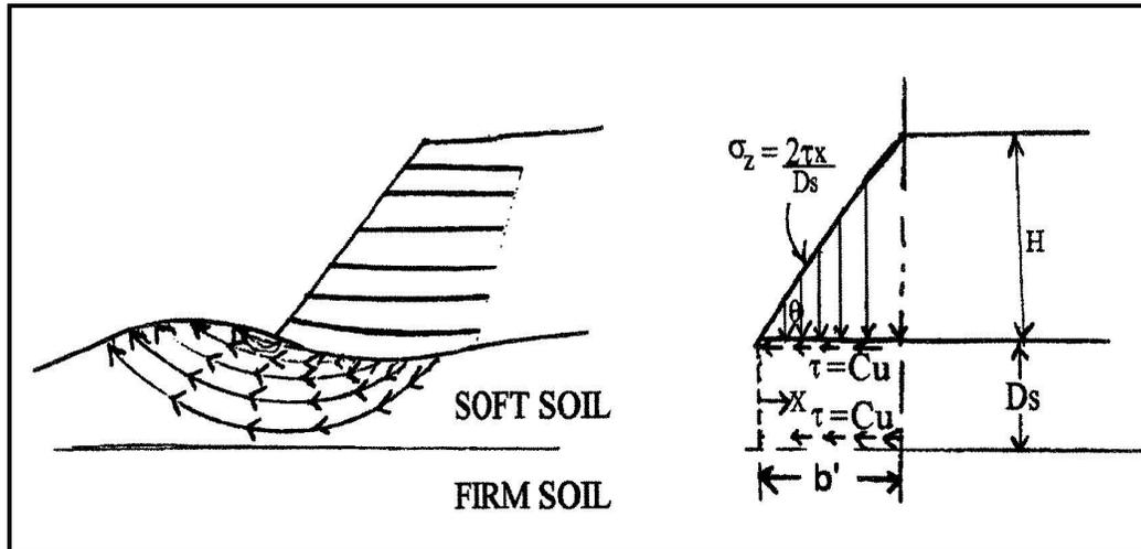
Figure D-13, Local Bearing Failure (Lateral Squeeze)
