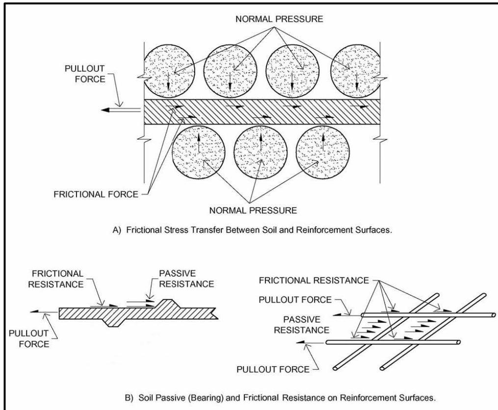
**Figure D-2, Mechanisms of Pullout Resistance
