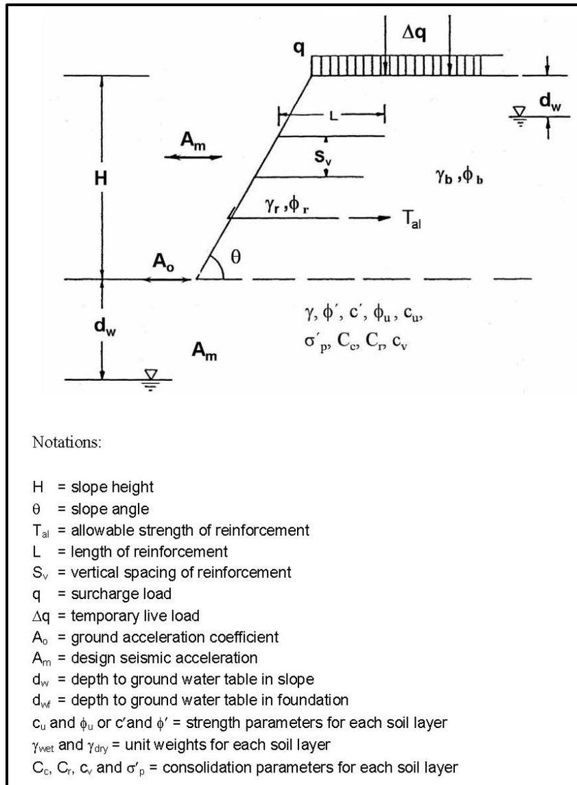
**Figure D-1, RSS Design Requirements and Geometry
