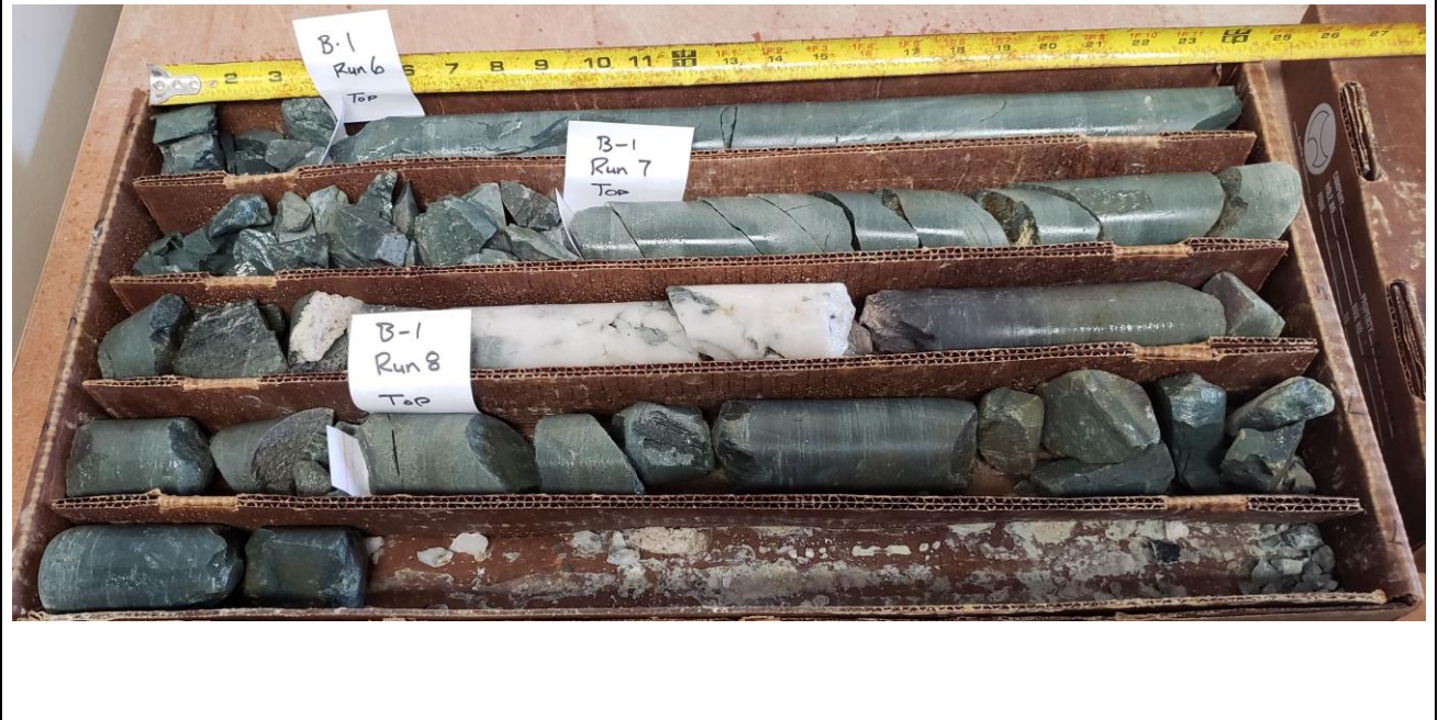
B-1 NQ-6: 33.7-35.1 feet; NQ-7: 35.1-40.1; and NQ-8: 40.1-43.1 feet
