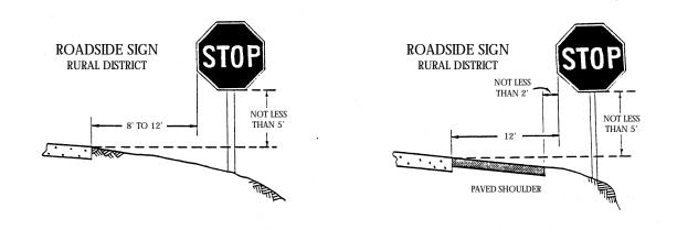
Figure 1A — Height and Lateral Location of Typical STOP Sign Insatllations
