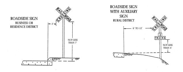
Figure 1B — Height and Lateral Location of Typical Crossbuck Sign Installations
