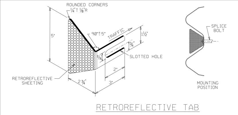
RETROREFLECTOR TABS SHALL BE 12 TO 14 GAUGE STEEL AND SHALL BE TRAPEZOIDAL (BUTTERFLY) REFLECTORS MANUFACTURED BY TAPCO OR APPROVED EQUAL.
