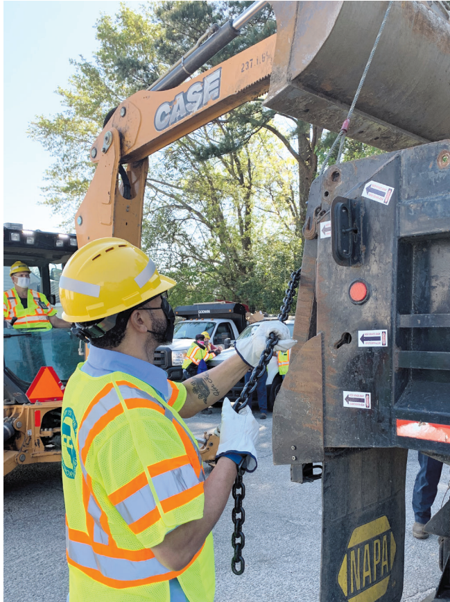
Orangeburg Maintenance employee Vincent Morris uses grade 80 chains to steady the tailgate while backhoe operator Randy Brunson lifts the tailgate.
