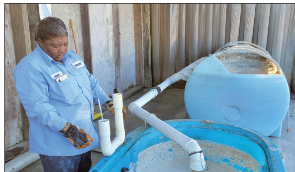
Brine making was being done around the clock to keep the roads treated. Here, Florence Maintenance makes the solution on Jan. 14, 2022.
