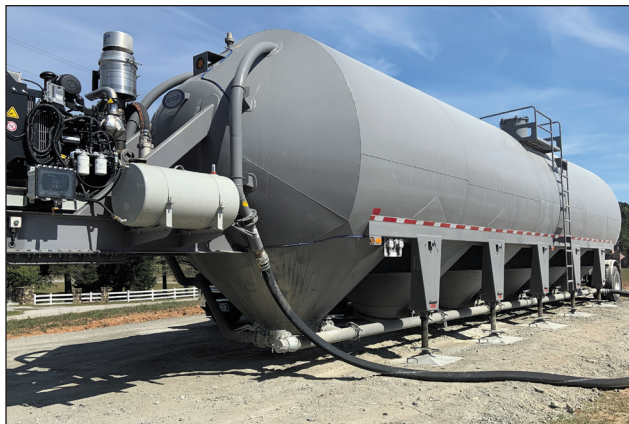
A powdered cement storage tank in Laurens County holds cement used in the process.
