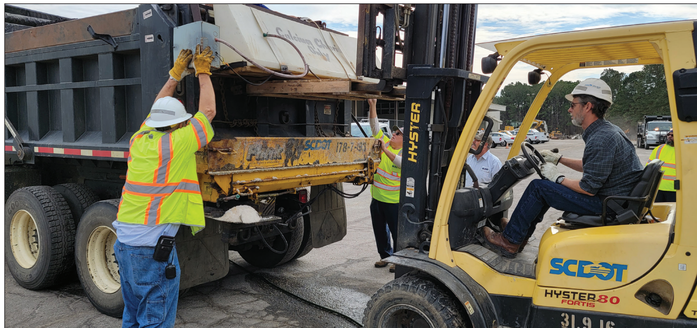
Horry Maintenance crews put a calcium chloride tank on the back of a dump truck to keep up with pretreating in the area on Jan. 20, 2022.
