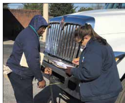
Resident Maintenance Foreman Henry Long and Foreman Dee Michaelson pull a stop bar measurement for a single-axle truck.
