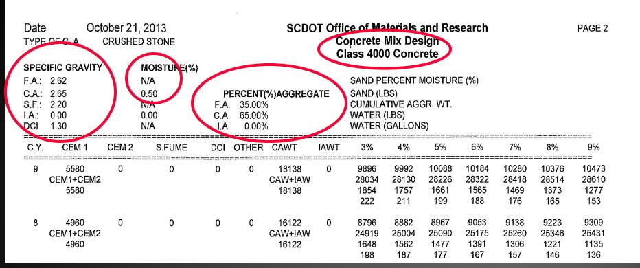
Class 4000 Concrete Specific Gravity of Aggregate Aggregate Proportion Coarse Aggregate Moisture
