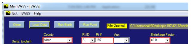
For the **Shrinkage Factor**, refer to the map area for the County to determine whether to use 30% or 40% unless otherwise directed by the Engineer of Record.
