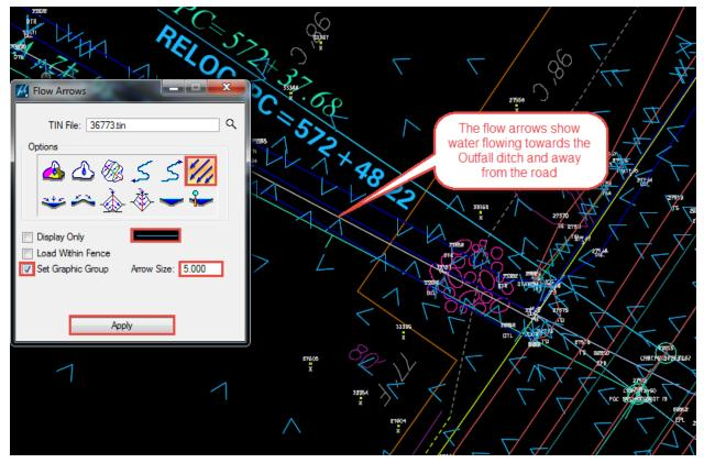
Select the **Ponds** Option and set the symbology as desired. Ensure **Fill** is turned on in the View Attributes. Turn on the Set Graphic Group and press the Apply button. Pan through the dtm file and review any ponding areas to look for during the design process, especially in intersections.
