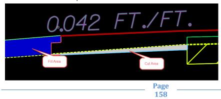
Turn OFF the RD\_XS\_EwShp level and select File > Save Settings (or Ctrl + F). This keeps the shapes from plotting on the cross section sheets.
