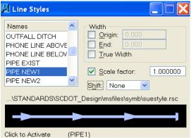
The line styles were developed for an English scale of 50:1. If using another scale, key-in the following values in the Scale Factor box of the line styles dialog.
