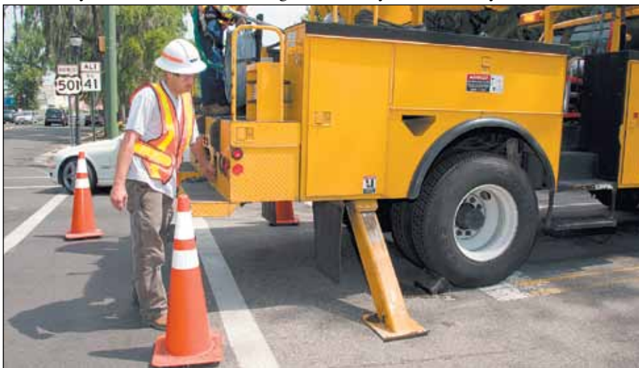
Ray Anderson of the District 5 Traffic Signal crew lowers the outriggers on the bucket truck.
