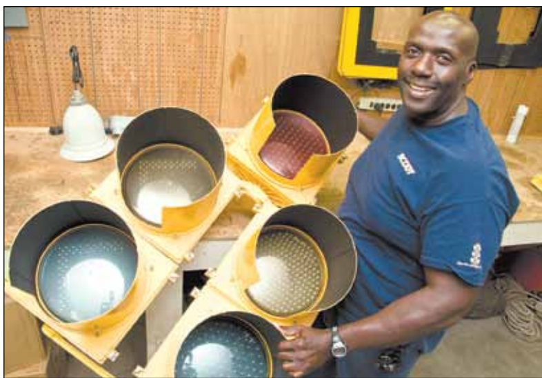
District 1 Traffic Signal Communications Manager Curtis Singleton is holds a 5-section traffic signal head. This head contains two left turn arrows. LEDs are replaced when they reach 60% burning due to bulb burnout. They are used for less power consumption. Standard incandescent uses 120W per bulb. These use 10-15W per head. A whole intersection now uses the power that use to power one single light.
