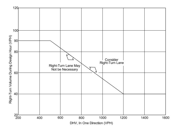
Note: Figure is only applicable on highways with a design speed of 50 miles per hour or greater.
