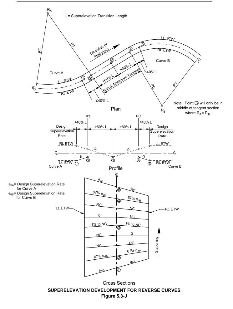
3. If the superelevation transition is located on the bridge or its approach slabs, coordinate with the structural designer. Typically, the designer should place on the roadway approach that portion of the superelevation development that transitions the roadway cross section from its normal crown to a point where the roadway slopes uniformly. This will avoid the need to warp the crown on the bridge or the bridge approach slabs.
