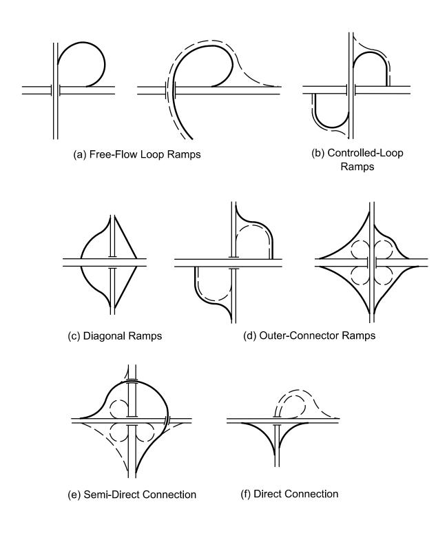
Note: The heavier solid line indicates the ramp type being addressed.
