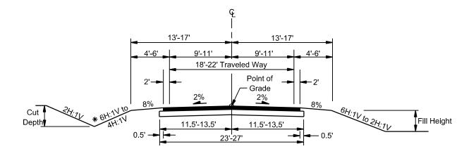
\*This slope may vary between a minimum slope of 6H:1V to a maximum slope of 4H:1V. Where a deeper ditch than provided by a 4H:1V slope is necessary for drainage purposes, continue the 4H:1V slope until the necessary depth has been obtained. This will place the ditch further from the roadway. Provide a separate profile for special ditch grades.
