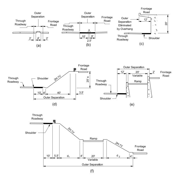
TYPICAL OUTER SEPARATIONS Figure 17.5-D SPACER PAGE
