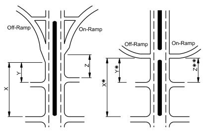
\* Measured from the end of the lane taper if an acceleration lane exists for the off-ramp.
