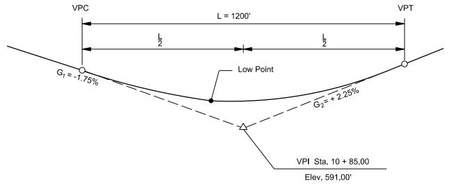
VPC Station = VPI Sta -  $\frac{1}{2}L = (10 + 85) - 600 = 4 + 85.00$ VPT Station = VPI Sta +  $\frac{1}{2}L = (10 + 85) + 600 = 16 + 85.00$
