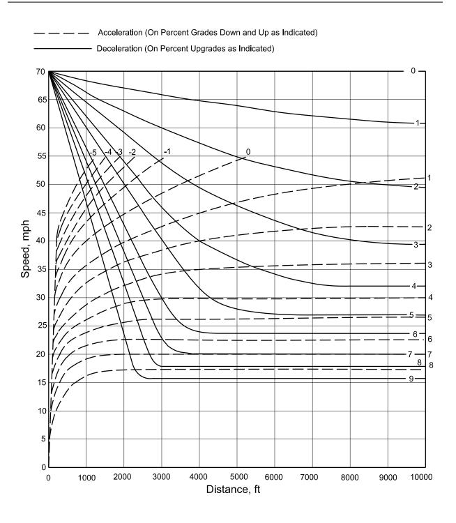
Note: For entering speeds equal to or greater than 70 miles per hour, use an initial speed of 70 miles per hour. For speeds less than 70 miles per hour, use the design speed or posted speed limit as the initial speed.
