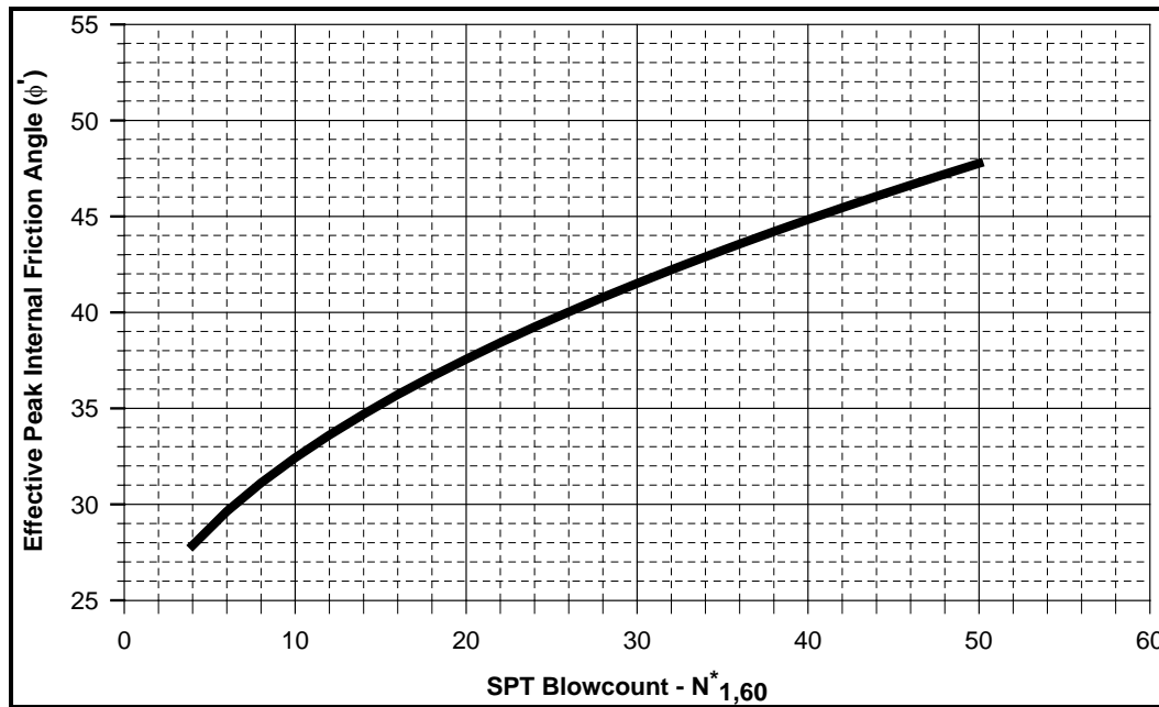
Figure 7-18, Effective Peak Friction Angle and SPT ( N_{1,60}^* ) Relationship (Based on Hatanaka and Uchida (1996))
