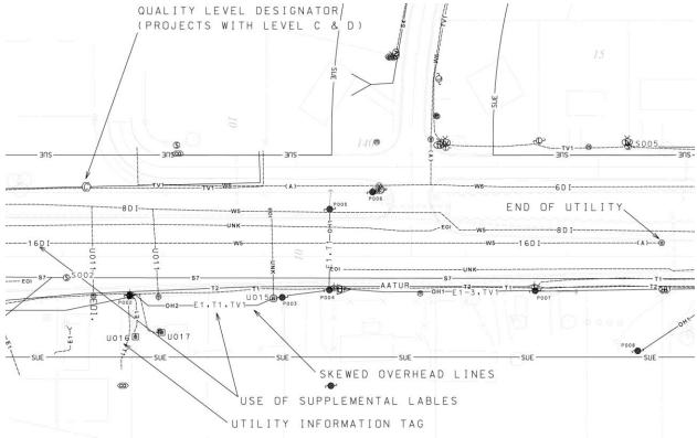
Figure 1 Supplemental Utility Line Label Example
