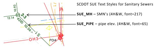
Figure 5 Sewer Manhole Number
