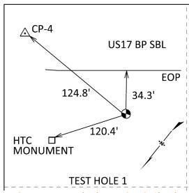
Figure 14 Test Hole Three Point Tie Sketch
