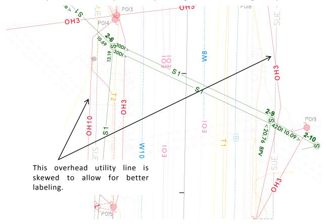
Figure 6 Overhead Utility Line-Work
